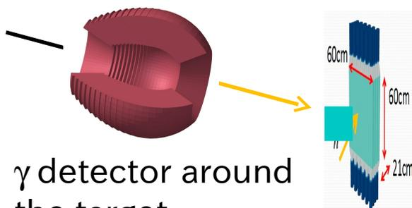
$\gamma$  detector around the target
