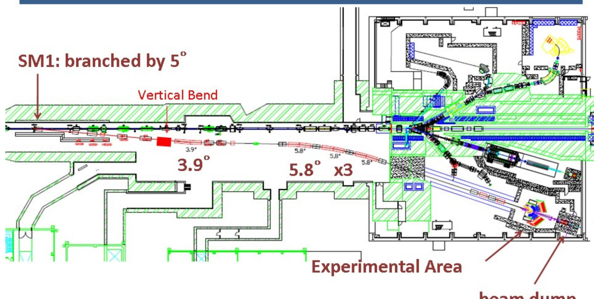
Beam dump and shields are for  $10^{10}$  protons/s
