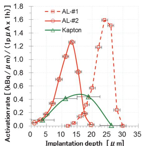
Fig. 1. Implantation-depth profile of thin-foil stacks.
