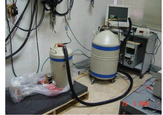
ULE-ULB-HPGe Prototype [20 g]
