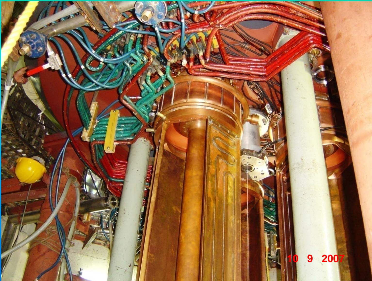
Lower outer conductor spinning assemblies
