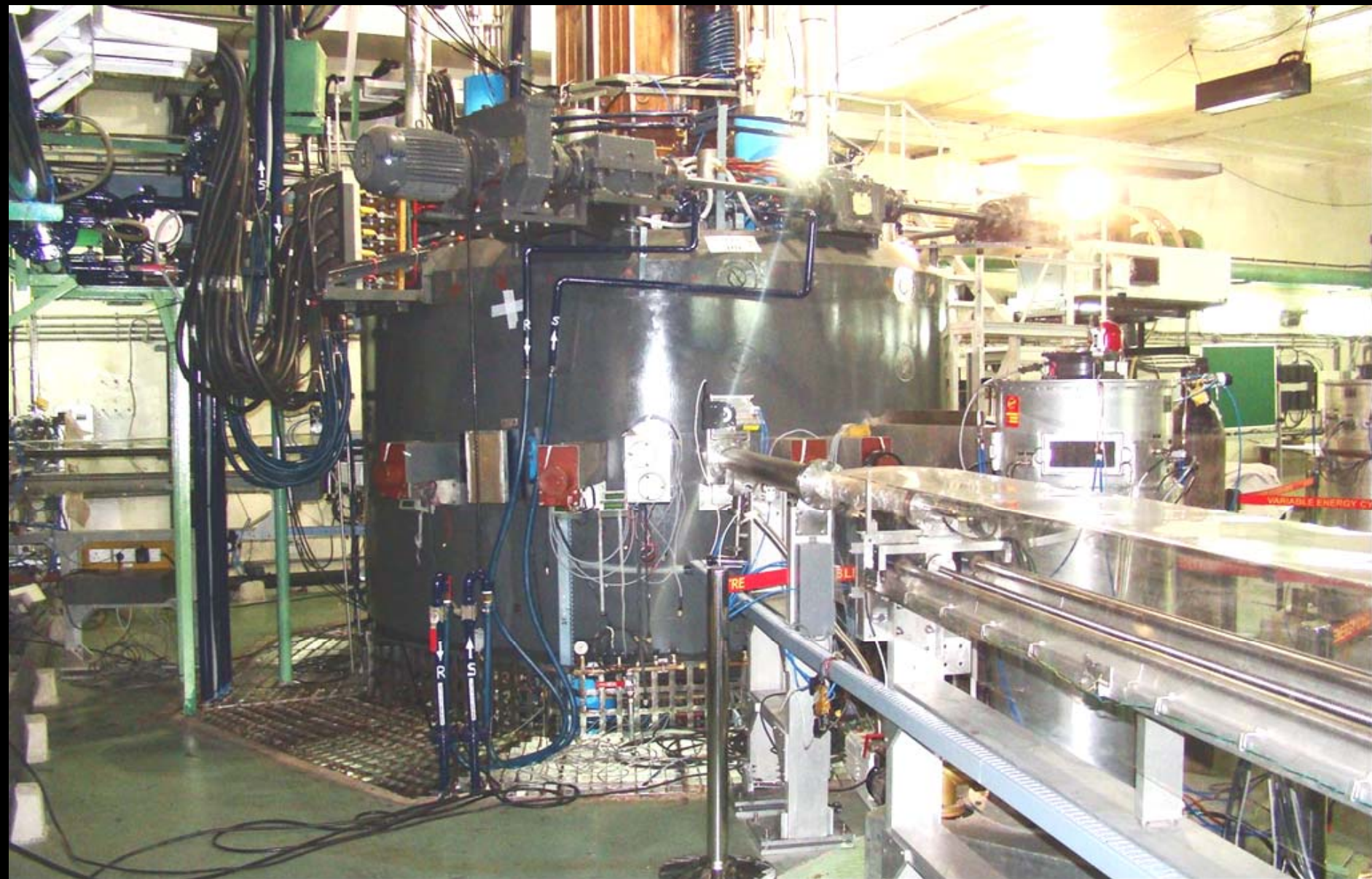
SUPERCONDUCTING CYCLOTRON WITH MAGNETIC CHANNEL AND MAIN BEAM PROBE DRIVES
