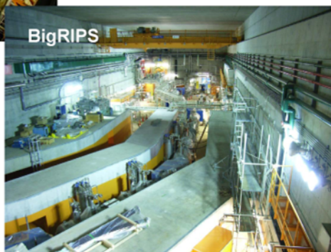
BigRIPS World's Largest Acceptance 9 Tm Superconducting RI beam Separator
