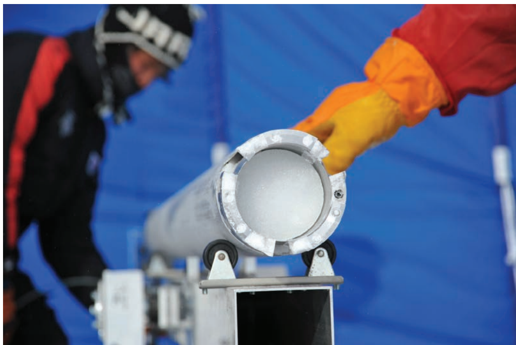
An ice core that has been drilled from near the Dome Fuji station in Antarctica.
