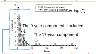
The histogram with the power lower than 40 is reproduced by the white noise. The components there may be caused by the fluctuation due to measurement uncertainties.
