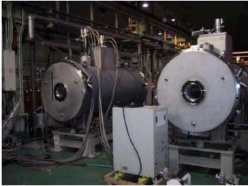
Superconducting quadrupole triplet(STQ):
