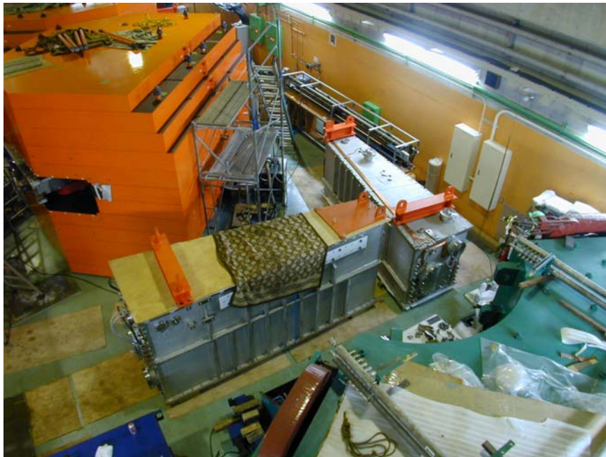
Figure 3.2.6. Main rf resonator of the fRC temporarily installed in the E4 experimental room. The resonator is divided into upper and lower parts.
