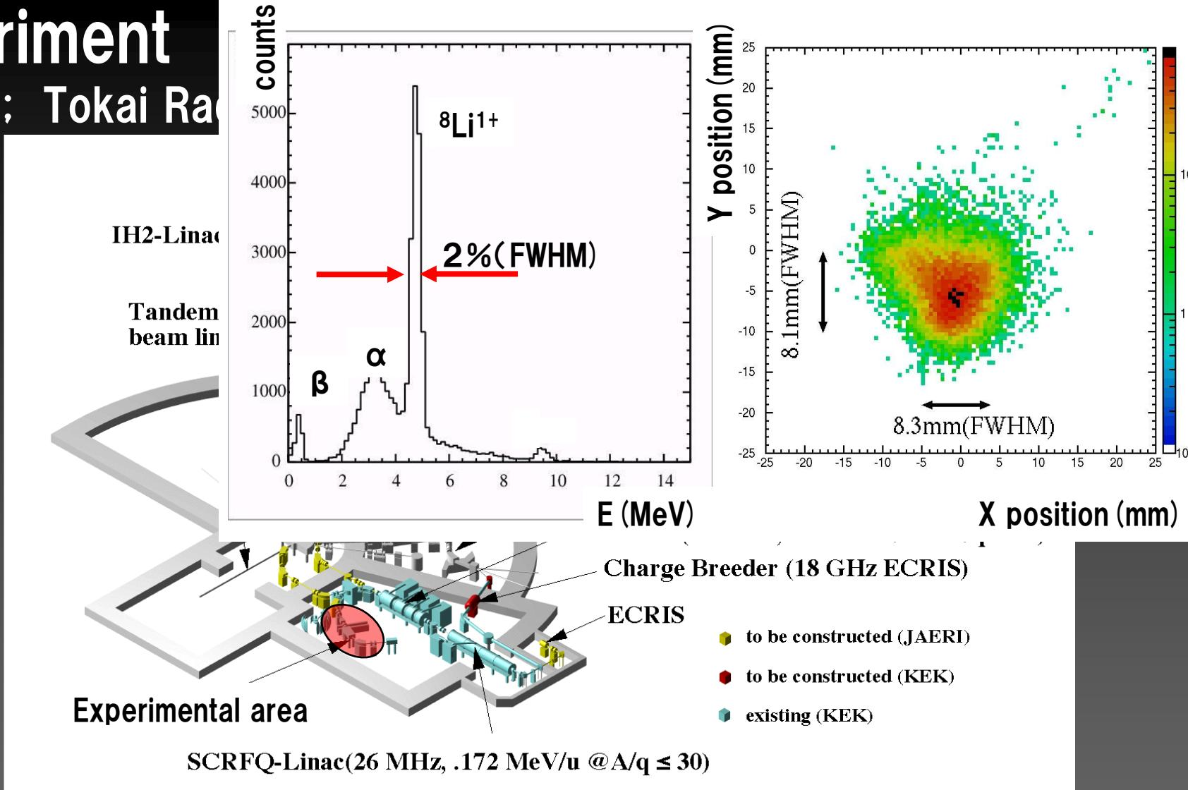
RNB can provide with variable output energy from 0.18 to 1.1 MeV/u
