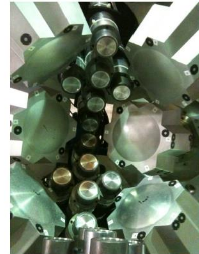
18 LaBr 3 (Ce) (1.5" x 2") 2 BC-418 Plastic 2mm thick Fast-timing measurements
