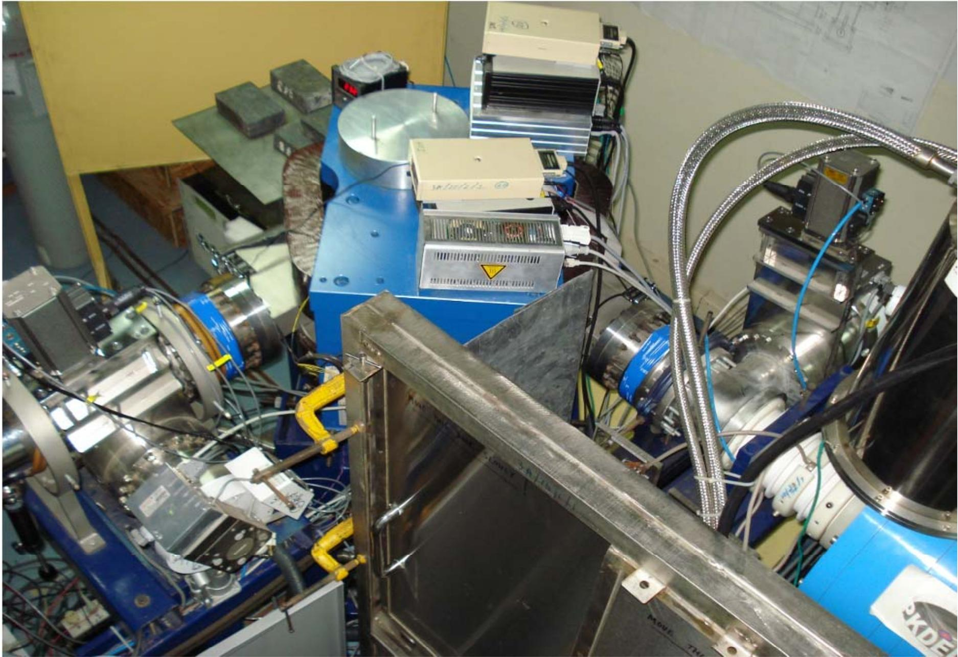
**World's first High Tc Superconductor based ECR source,
