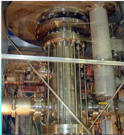
45 Tesla : strongest steady magnetic field (High Mag. Field. Lab. In Florida)
