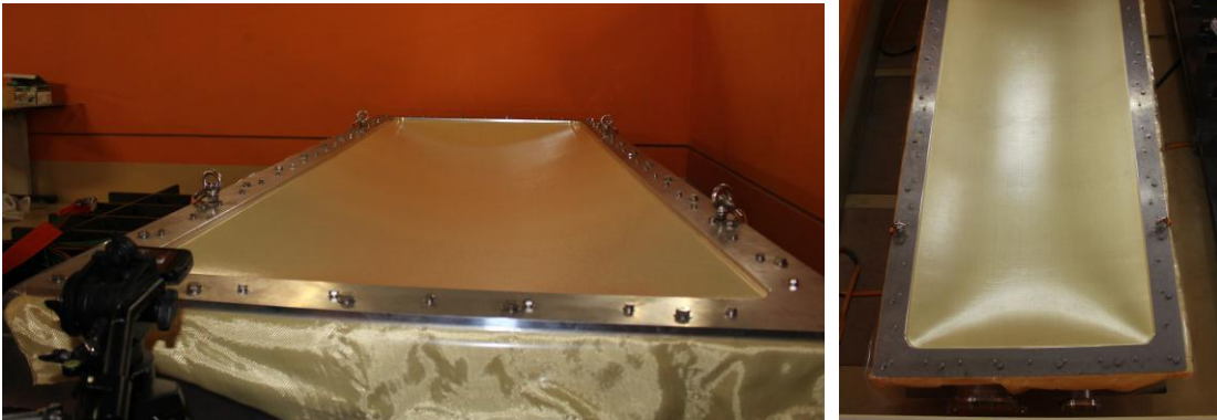
Fig. 2-3-7: Shape of the vacuum window at 100 mbar. Distance to the deepest face is about 20 cm.
