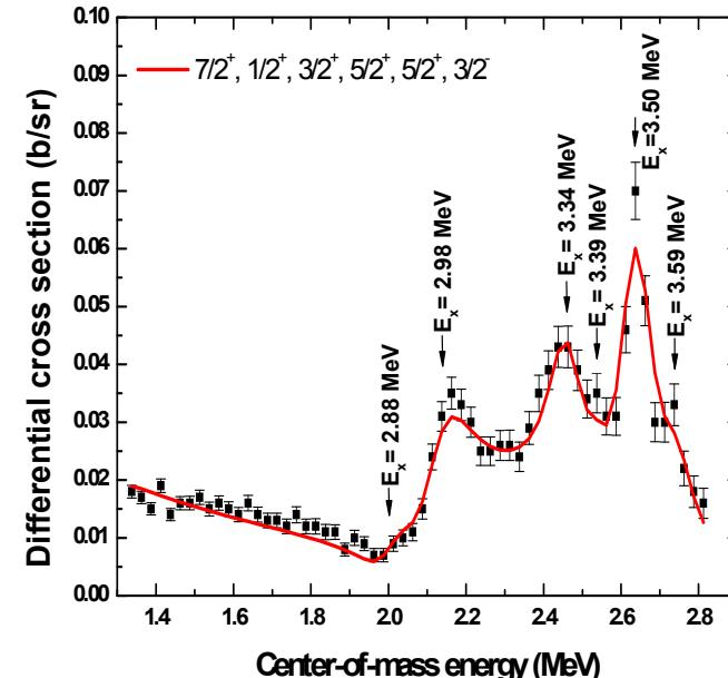
$^{26}\text{Si} + \text{p}$  experiment: Observed proton resonances with resonant scattering, and determined resonance parameters:
